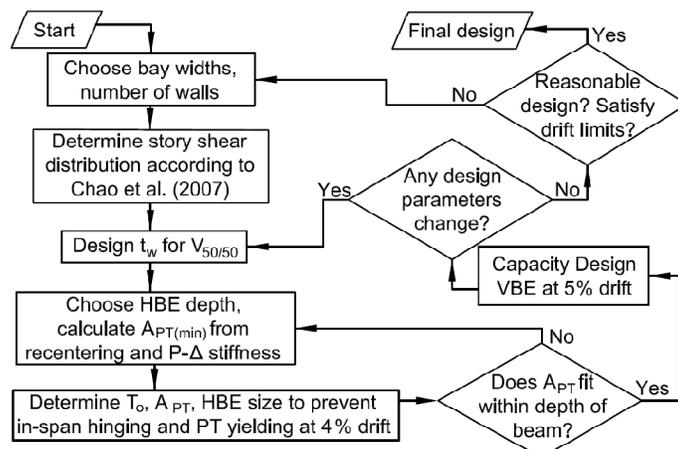
Fig. 4: SC-SPSW performance-based design procedure
