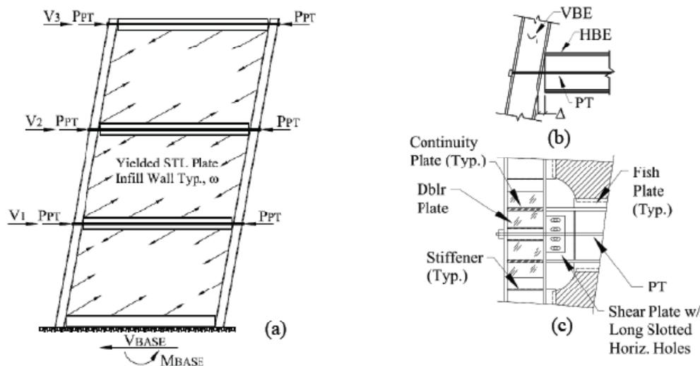
Fig. 1. SC-SPSW: (a) Yield Mechanism; (b) rocking joint; (c) rocking detail
