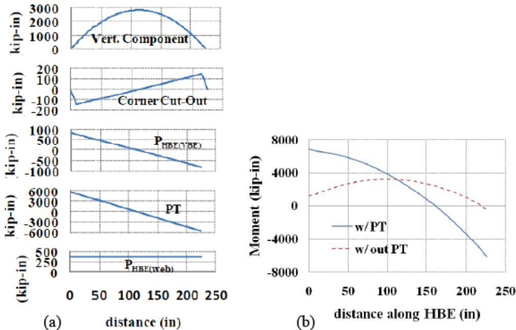
Fig. 3. (a) HBE Moment Components (b) Composite Moment Diagram
